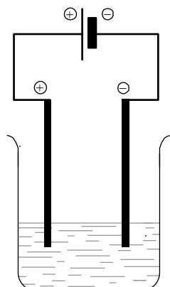
electrolytic cell showing solid electrodes immersed in solution;
